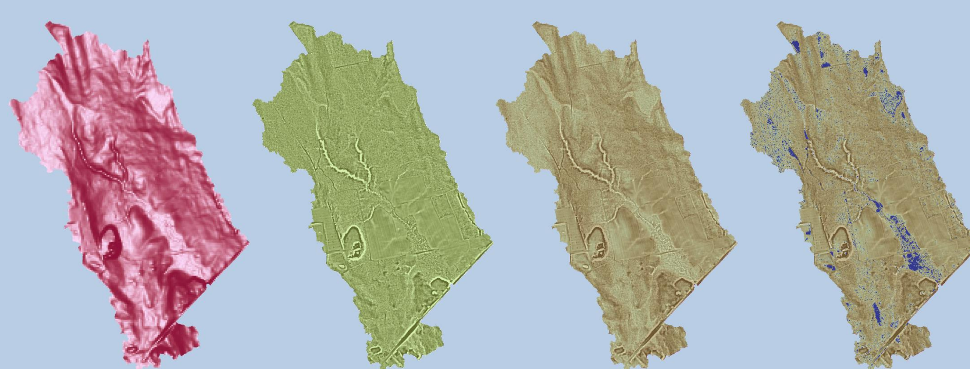
Figure 5. LiDAR derivative layers showing slope (low-high: light-dark purple), TPI (low-high: light-dark green), and slope-TPI visual overlay (lightest browns are flattest slopes and lowest TPIs), plus overlay with storage
